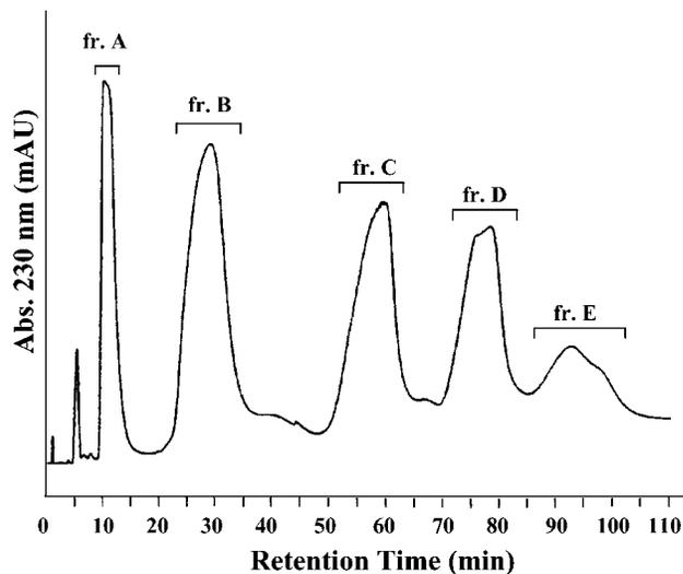
**Figure 2.** Profile of apple procyanidins separated by normal phase chromatography using a mixture of hexane and acetone as the mobile phase. The eluate was monitored by an absorbance at 230 nm. Fractions: A, flavan-3-ol fraction; B, procyanidin dimer fraction; C, procyanidin trimer fraction; D, procyanidin tetramer fraction; E, procyanidin pentamer fraction.
