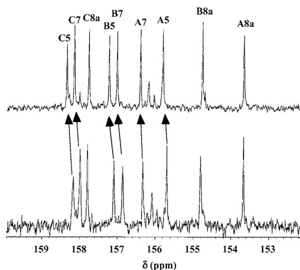
**Figure 6.**  $^{13}\text{C}$  NMR spectra of procyanidin C1 in  $\text{CD}_3\text{OH}$  (A) and  $\text{CD}_3\text{OD}$  (B) at  $-20^\circ\text{C}$ .
