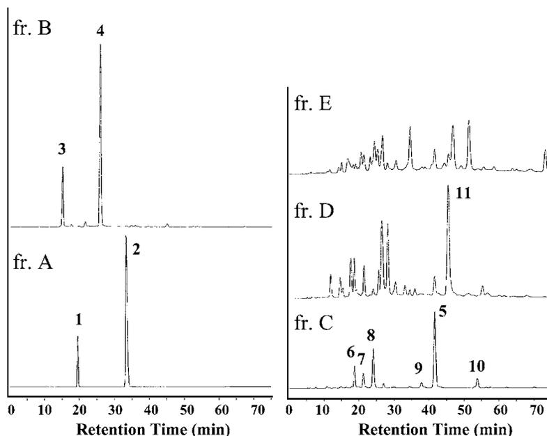
**Figure 3.** Reversed phase HPLC profiles of apple procyanidins fractions (A–E) separated by normal phase chromatography. Peaks: 1, (+)-catechin; 2, (–)-epicatechin; 3, procyanidin B1; 4, procyanidin B2; 5, procyanidin C1.
